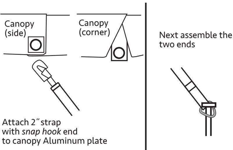
Attach 2" strap with snap hook end to canopy Aluminum plate
